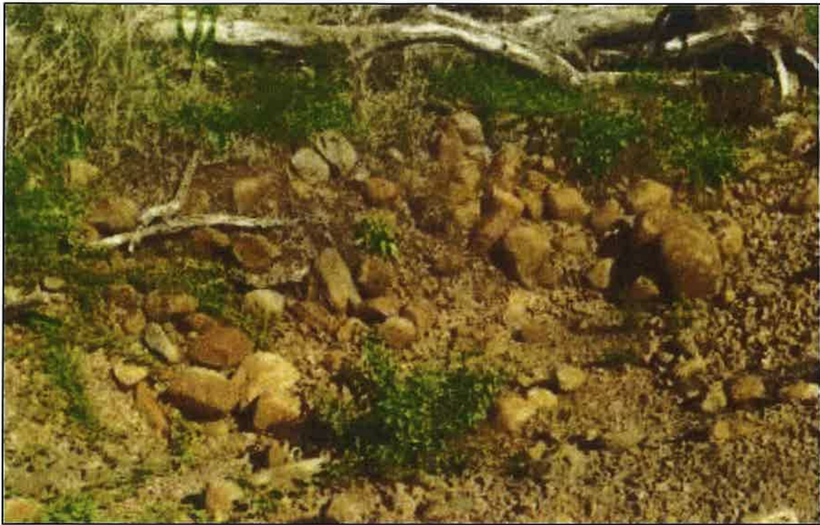
Figure 5: Colluvium – Predominantly Soils with Basalt Cobbles
